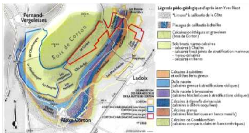
Fig1 : The different soil and limestone layers in the “Colline de Corton” area (J.Y. Bizot, 1992)
