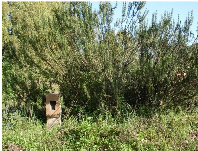
Figure 3: Camera as installed in the field. Camera is hidden in wooden beam that has been hollowed out. Two pieces of plywood are used to enclose the camera (with detection surface removed). NB: Case is still to be painted dark brown for optimal camouflage.
